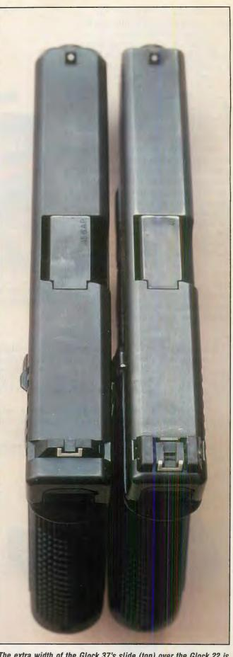
The extra width of the Glock 37's slide (top) over the Glock 22 is apparent here. This requires a different holster. The .45 GAP (on the left) uses a rebated, rimless case, preventing the .45 ACP from being interchanged with it.
